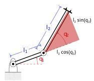
We know that the base of this triangle is  $l_2cosq_2$  while the height of the triangle is  $l_2sinq_2$
