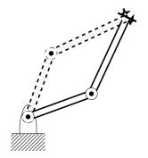
The inverse kinematic model might have more than one solution for a specific pose
