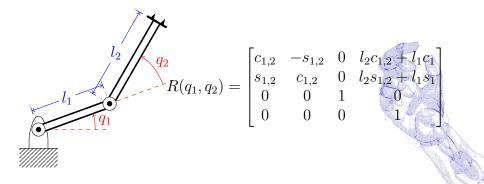
$$\begin{bmatrix} c_{1,2} & -s_{1,2} & 0 & l_2 c_{1,2} + l_1 c_1 \\ s_{1,2} & c_{1,2} & 0 & l_2 s_{1,2} + l_1 s_1 \\ 0 & 0 & 1 & 0 \\ 0 & 0 & 0 & 1 \end{bmatrix} = \begin{bmatrix} X_X & Y_X & Z_X & P_x \\ X_Y & Y_Y & Z_Y & P_y \\ X_Z & Y_Z & Z_Z & P_z \\ 0 & 0 & 0 & 1 \end{bmatrix}$$
