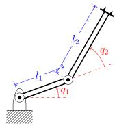
For the second segment, we think alike.  $P_2(q, \dot{q}) =$  $m_2g\left(l_1sinq_1 + \frac{l_2}{2}sin(q_1 + q_2)\right)$ The total potential energy is therefore:  $P(q, \dot{q}) = m_1 g \frac{l_1}{2} sinq_1 + m_2 g \left( l_1 sinq_1 + \frac{l_2}{2} sin(q_1 + q_2) \right)$
