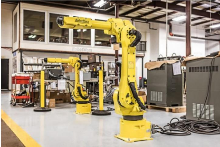
By controlling the position of the joints, we can control the position of the end-effector.
