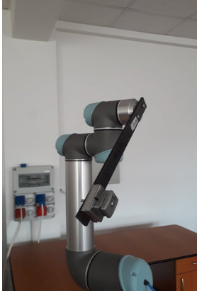
Fig. 3. Added mass off the axis of rotation, used for the identification of joint 4, 5, and 6
